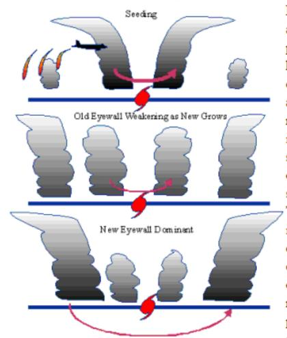
Project STORMFURY was an ambitious experimental program of research on hurricane modification carried out between 1962 and 1983. The proposed modification technique involved artificial stimulation of convection outside the eyewall through seeding with silver iodide. The invigorated convection, it was argued, would compete with the original eyewall, lead to reformation of the eyewall at larger radius, and thus, through partial conservation of angular momentum, produce
