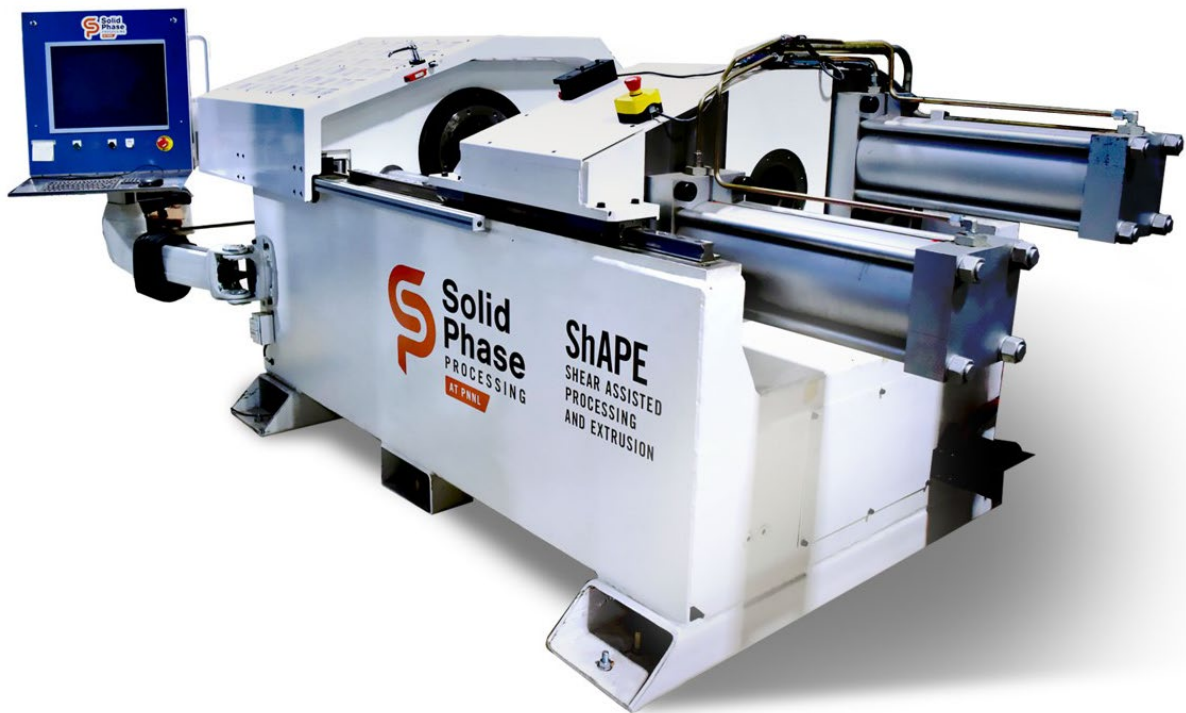
Figure 2. First-of-its-kind ShAPE machine installed in PNNL's Solid Phase Processing Laboratory. Source: PNNL
