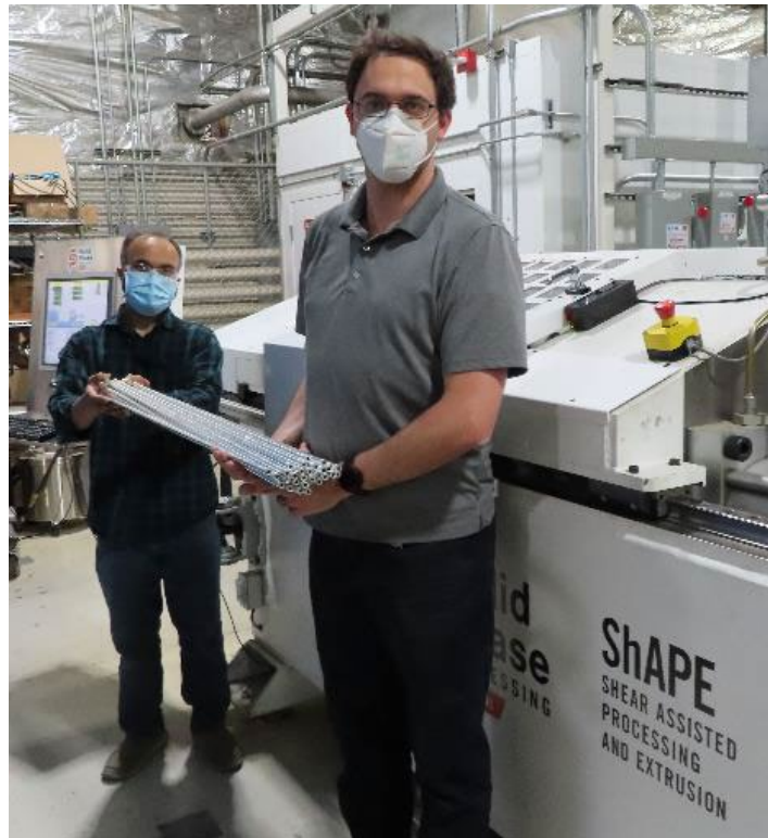
Figure 6. Bundle of ShAPE extruded Al 6063 tubing with 12 mm OD and 2 mm wall thickness. Source: PNNL.
