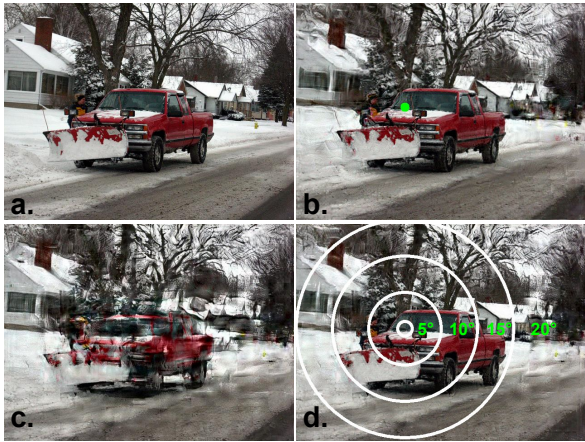
Figure 2: Original vs. Uniform Texture Tiling Model (TTM) . An original image (a) can be processed using the Original TTM (b) which is foveated, meaning that information is pooled in regions that grow farther from an assumed fixation point (green dot). To create our dataset we adapt TTM to use a fixed uniform pooling region size everywhere in the image, shown in (c) at 15^\circ eccentricity. We can efficiently stitch together multiple uniform TTM images from our pre-computed dataset to recreate the foveated effect (d).
